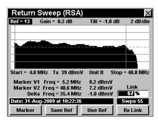
The 860 DSPi, with an SR-1 Option, injects an agile sweep signal configured to "step around" active channels, sweeping in unoccupied spectrum areas to a frequency resolution of 100 kHz. The reverse sweep is received by the 8310 RSA™ and the response information is relayed back to the 860 DSPi on via user configurable frequency agile forward telemetry signal.
